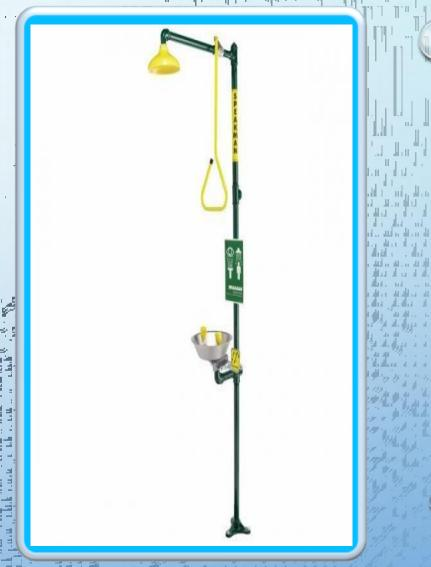
COMBINATION SHOWER WITH SE-693 EYEWASH WITH DUAL AERATED SPRAY OUTLETS, FUP TOP DUST COVERS AND STAINLESS STEEL BOWL: PAINTED GALVANIZED STEEL STANCHION WITH AN MPELLERACTION DELUGE SHOWER HEAD ACTIVATED BY A HIGH VISIBILITY YELLOW PULL ROD.
