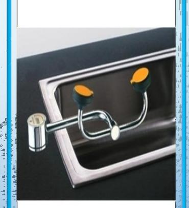
APPLICATION: AUTOFLOW EYE/FACE WASH FOR MOUNTING ON COUNTER NEXTTO SINK. SWINGING THE SPRAY HEAD ASSEMBLY 90 DEGREES HORIZONTALLY OUT OVER SINK ACTIVATES THE WATER FLOW. THE UNIT REMAINS IN OPERATION UNTIL THE SPRAY HEAD ASSEMBLY IS SWUNG BACK INTO THE STORAGE POSITION, CLOSING THE VALVE.
